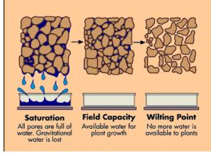
• Field capacity is detected within AquaSpy by looking for the inflection point, or change in slope, between free moving water and water being held in the pore space. This is best detected after a large rain or watering event where the soil is saturated.
