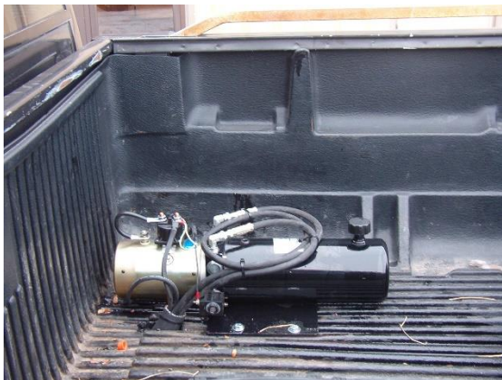
Power unit mounted in box
