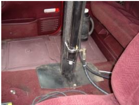
Inside mounting example, rubber dust seal.
